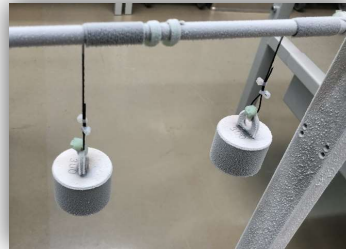
Figure 4 ESCC 3901 Para 9.17 Cold bend Test variant 14 sample after -80°C exposure
