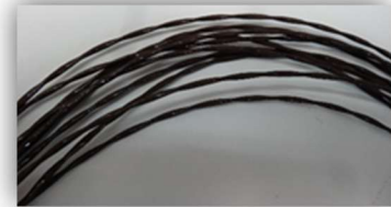
Figure 5 ESCC 3901 Para 9.28 Long Term Aging Test variant 14 sample after 2000h at 230°C
